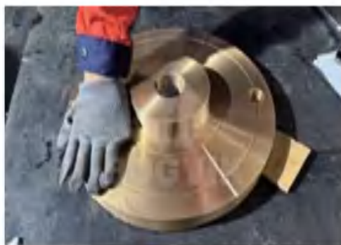
Main Shaft Step Bearing
